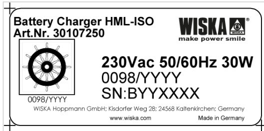
Figure 6 Nameplate Battery charger
